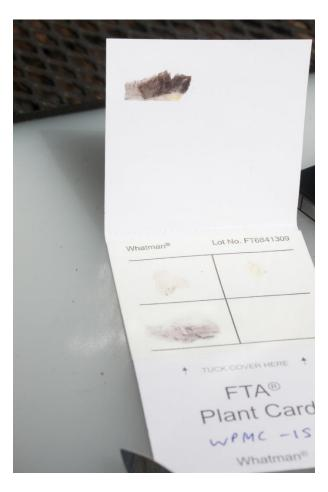
Figure 5 Remove any remaining material from the cover and very carefully from the filter paper.
