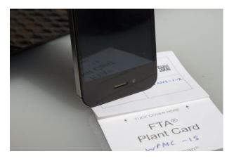
Figure 3 Squash the sample either with a hammer blow or by squeezing a hard object over it.
